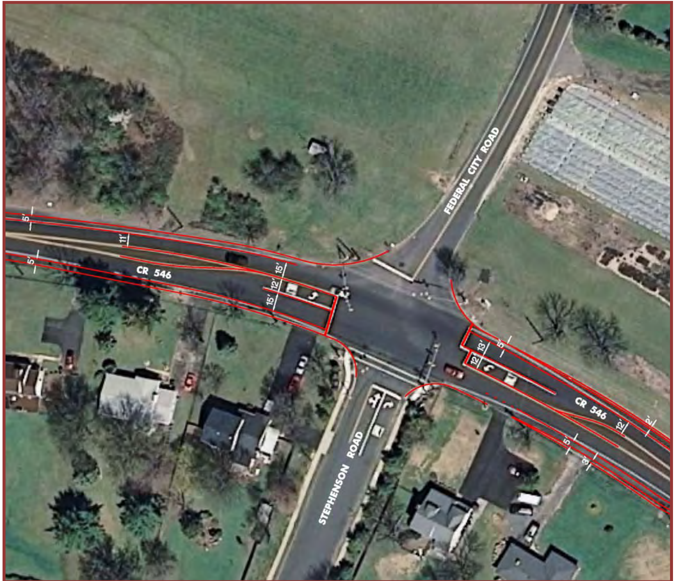
Figure 5: Concept #1 – Bicycle Lanes on CR 546 Intersection Striping CR 546 and Federal City Road/Stephenson Road
