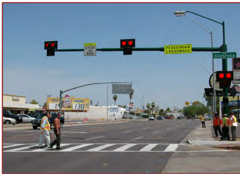
Example of a Pedestrian Hybrid Beacon
