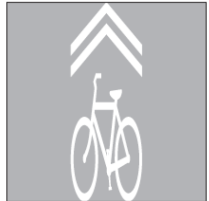
Shared lane marking MUTCD Fig. 9C-9
