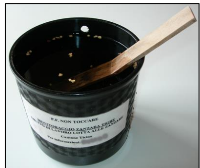
Above: The Ovitrap is a tool for the detection of Asian Tiger Mosquitoes.
