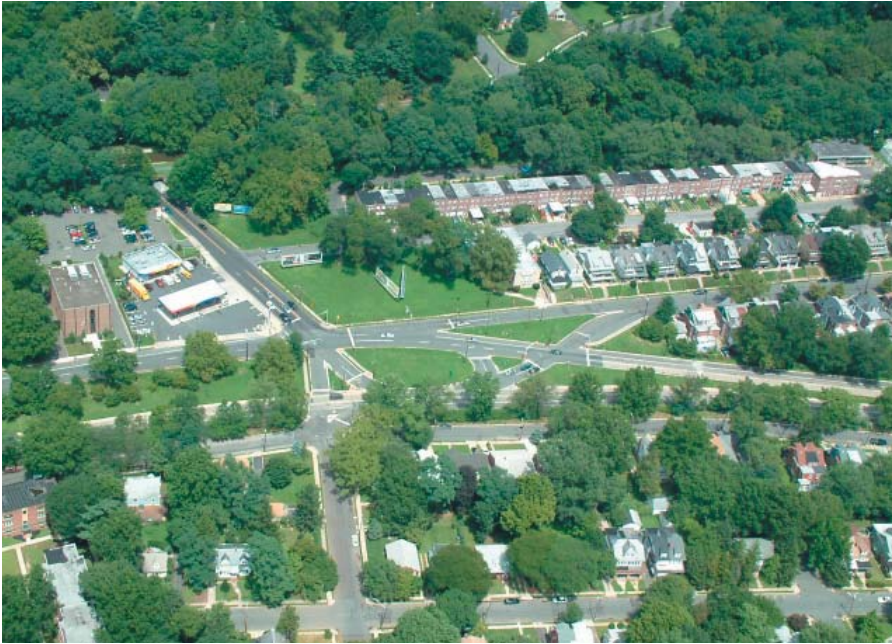
The wide median and complicated turning routes at the Sullivan Way intersection with Route 29.
