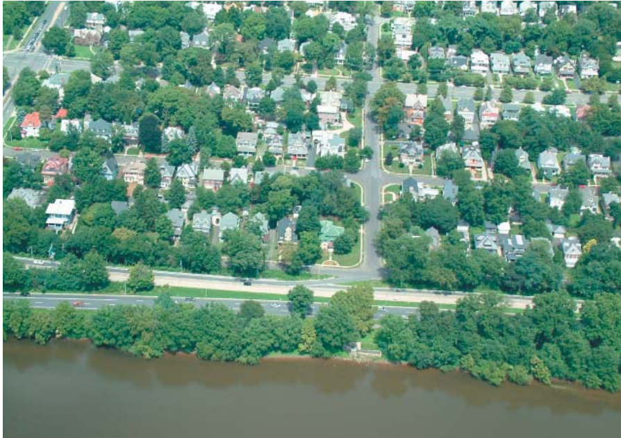
High speed slip ramps, such as the one at the base of Gouverneur Avenue, allow access to the neighborhood from Route 29 but encourage speeding.
