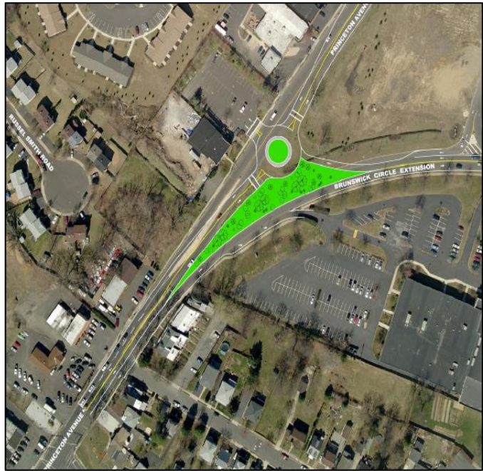
Proposed roundabout to replace the existing intersection
